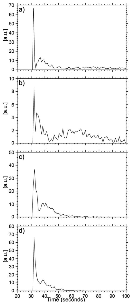
Fig. 3 Total ion current as a function of time for 2-NPG matrix-assisted ionization of insulin using (a) tapping, (b) 1 valve pulse, (c) 2 pulses and (d) 5 pulses at 1 Hz repetition starting at 30 s.
