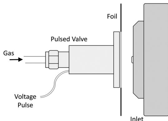
Fig. 1 Pulsed valve matrix assisted ionization schematic.
