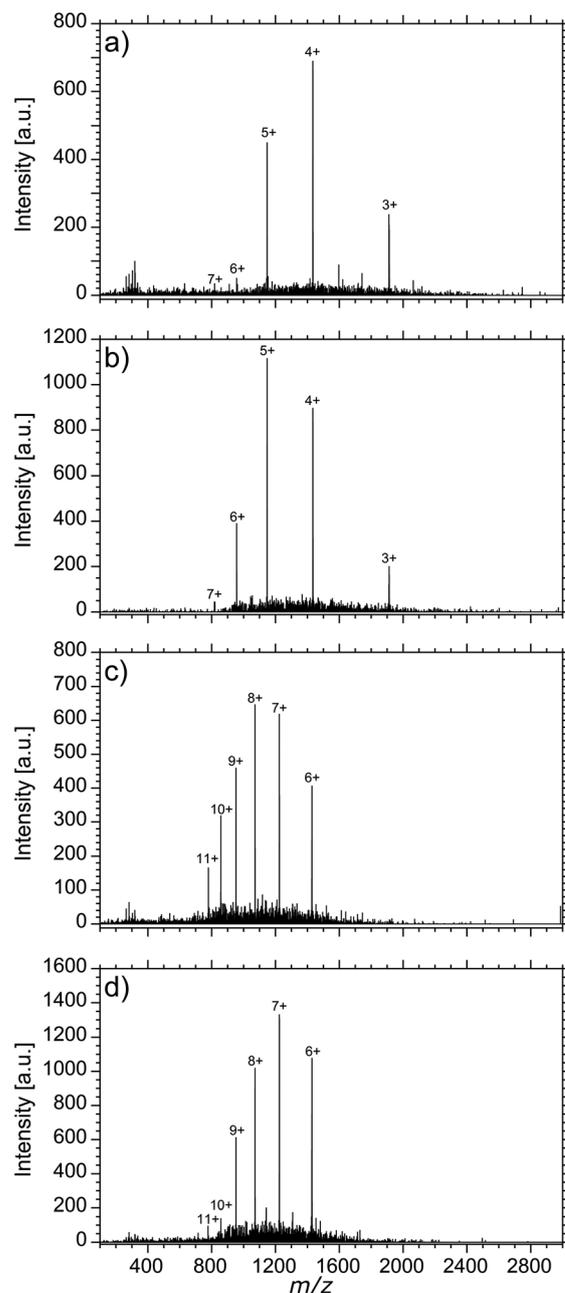
Fig. 2 Mass spectra for 2-NPG matrix-assisted ionization of (a) insulin using tapping, (b) insulin using pulsed valve and (c) ubiquitin tapping, and (d) ubiquitin with pulsed valve.
